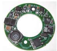
Custom low voltage “embedded” LED Driver
