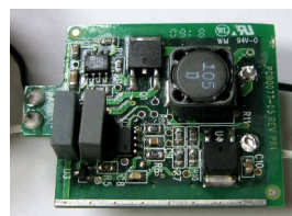
Custom 120VAC LED “embedded” Driver
